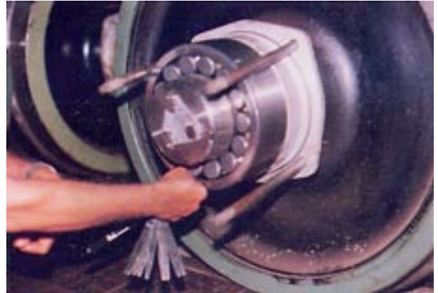
Fig 19 Checking Brg. radial clearance in mounted condition
